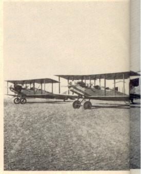
was the most plentiful design around at the time. The Swallow did owe much to the Jenny, differing most notably in having a round instead of straight-side nose radiator, equal-span wings, and a side-by-side, two-seat cockpit.
